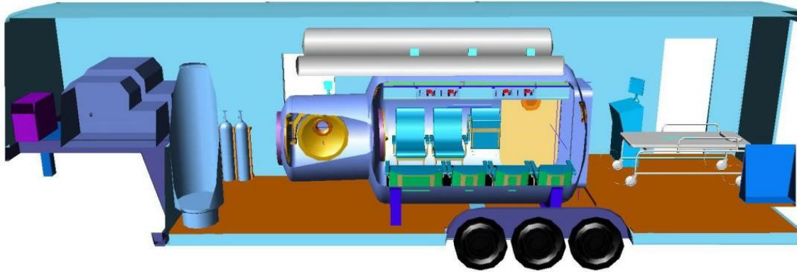
Dual Lock Chamber Layout - 6 place, 84" Diameter
